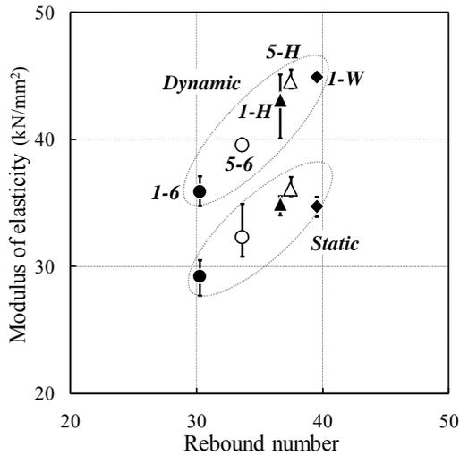
Figure 5. Relationships of rebound number to static or dynamic modulus of elasticity
