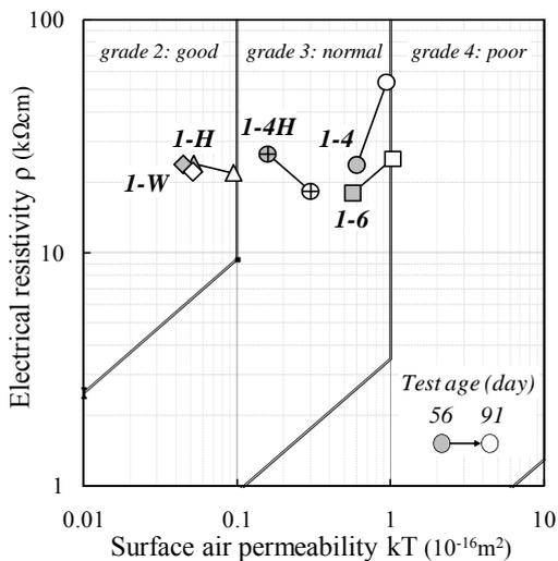
Figure 9. Effects of exposure condition on electrical resistivity and surface air permeability of the specimens demolded at one-day age
