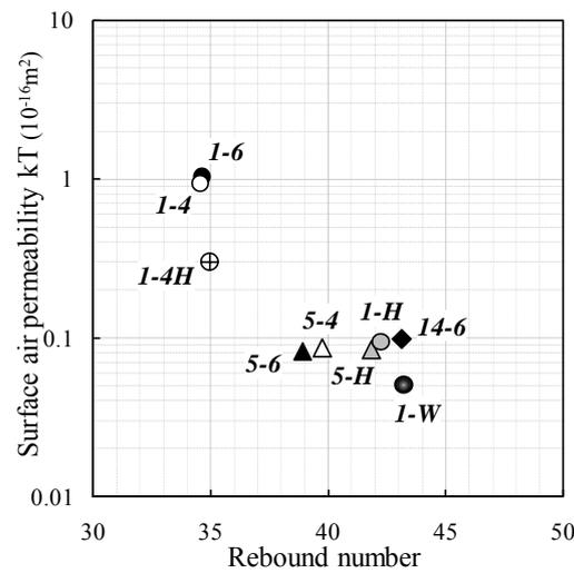
Figure 13. Relationship between surface air permeability and rebound number measured at 91-day age for all the specimens
