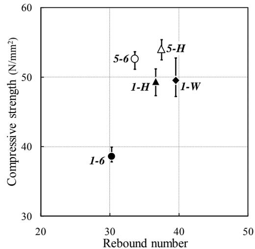
Figure 4. Relationships between rebound number and compressive strength
