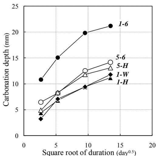
Figure 14. Relationship between duration of acceleration and carbonation depth
