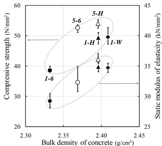
Figure 2. Relationships of compressive strength or static modulus to elasticity and bulk density
