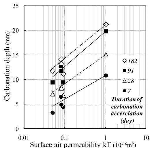
Figure 15. Relationship of carbonation depth to surface air permeability at 91-day age
