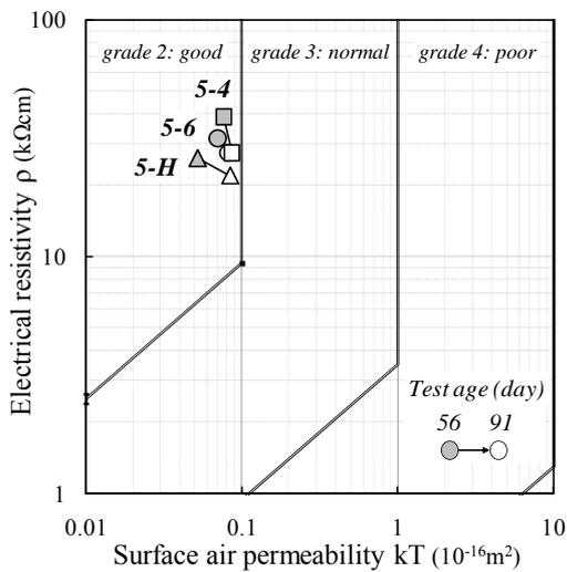
Figure 7. Electrical resistivity and surface air permeability of the specimens demolded at five-day age
