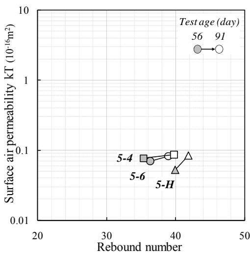
Figure 10. Relationship between surface air permeability and rebound number of the specimens demolded at five-day age
