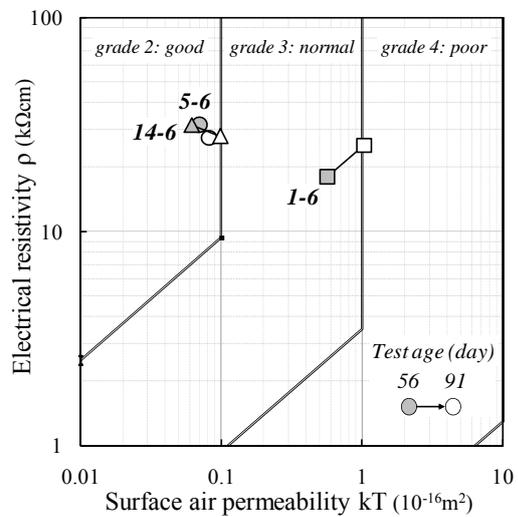
Figure 8. Effects of demold age on electrical resistivity and surface air permeability of the specimens exposed to 60%RH air
