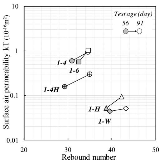
Figure 12. Effects of exposure condition on surface air permeability or rebound number of the specimens demolded at one-day age
