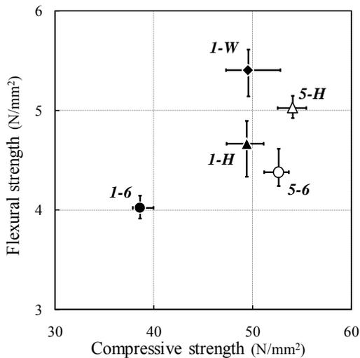
Figure 3. Relationships between compressive and flexural strength
